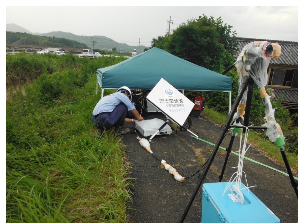
Real time observation by a satellite communication equipment(Ku-SAT II)
