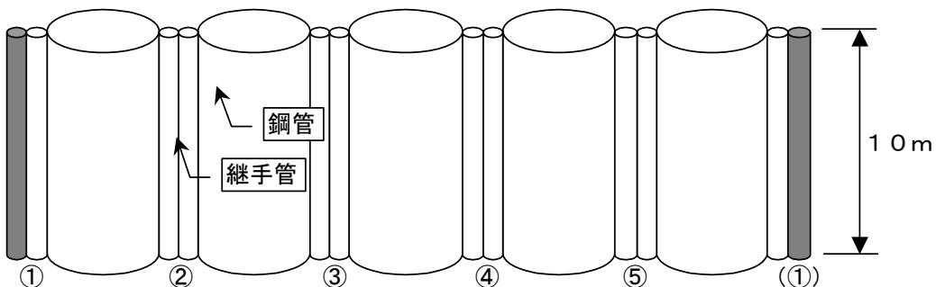
$$\text{継手管延長} \times \text{継手箇所数} \\ 10\text{m} \times 5 \text{箇所} = 50\text{m} \quad \therefore \text{積算数量} = 50\text{m}$$
