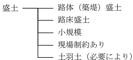
$$※ \text{ 土羽土 } V (\text{m}^3) = A (\text{m}^2) \times 0.3 (\text{m})$$
